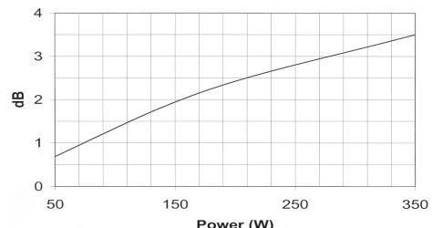
Note: These losses are calculated from a five minutes AES power test applying band limited pink noise (120-3500 Hz). The loudspeaker is free-air standing.
